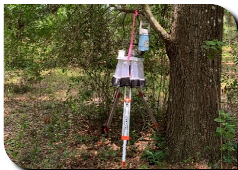
Picture 21: Rotator trap to identify times of peak mosquito flight activity
