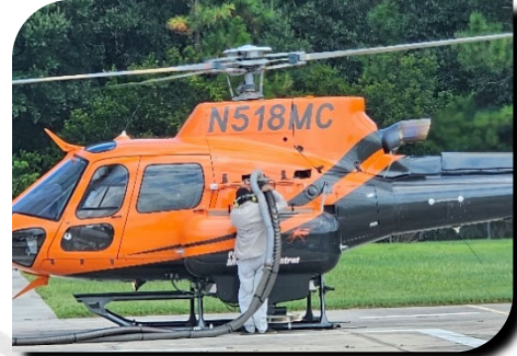
Picture 6: Treatment material filling hopper on helicopter
