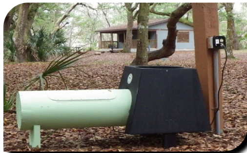
Picture 20: Suction trap used to collect adult mosquitoes
